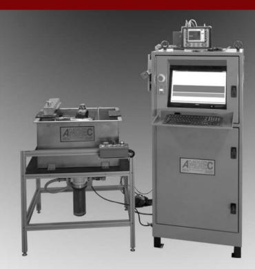
Over many years, a variety of Andec's in-house-developed Ultrasonic Laserweld Inspection Technology (ULIT) systems, have been installed in many automotive assembly welding lines. They are available with robotic or overhead pick and place, load/unload, or, manually, with surround guarding and safety light curtains.
